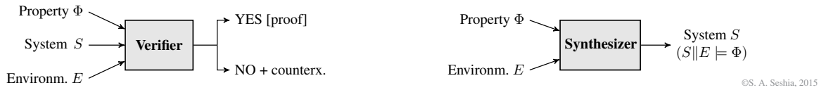
Figure 1: Illustration of formal verification and synthesis: A verifier generates as output a YES/NO answer, indicating whether the systems S satisfies the property \Phi in its environment E ; In contrast, a synthesizer generates a system model S from a class of systems that satisfy \Phi when composed with E .
